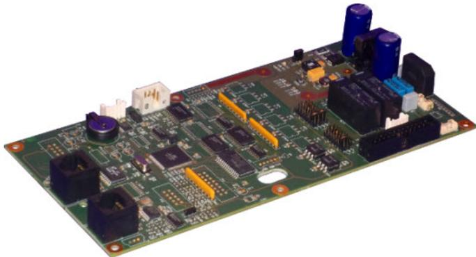
**Our Parking Machine Control board is design to connect all the components needed to make a fixed free parking machine.**
