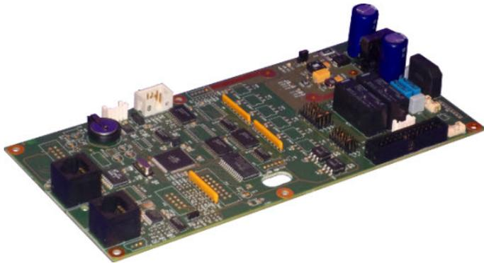
**Our Coin Payment Solution control board V2, has been design to connect all the components needed to make a fixed free payment systems for pedestrian turnstiles and gates.**
